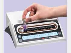
Return activated BI to color-coded incubation well. Observe LCD panel to confirm BI is correctly seated. Remaining incubation time, in minutes, will be displayed directly below BI on the LCD display to indicate incubation is in progress.
