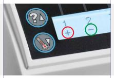
Observe LCD panel under incubating Bls for negative (–) or positive (+) result. The positive control should read positive (+). A positive result for a test (processed) Bl, which indicates a sterilization process failure, should be acted upon immediately.
